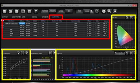
check the bits at corresponding positions of those data, can also go to "Settings" page to add the custom benchmark light source, and compare with the Lighting Passport measurement data.
